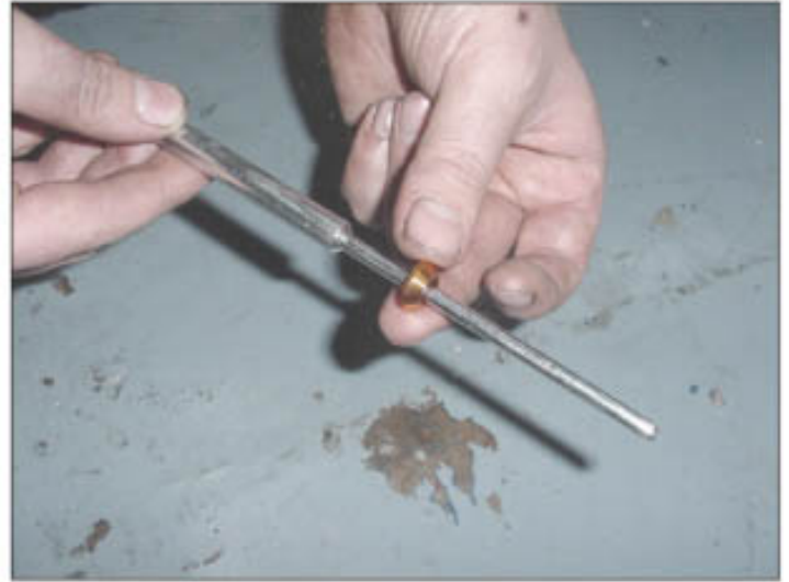
Figure 14 – Using Extractor Tool pin to guide copper packing
