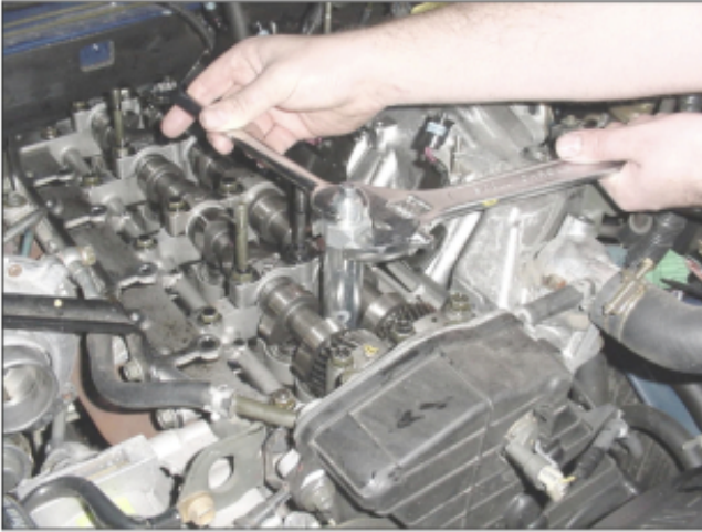
Figure 8 – Extracting the sleeve using the tool
