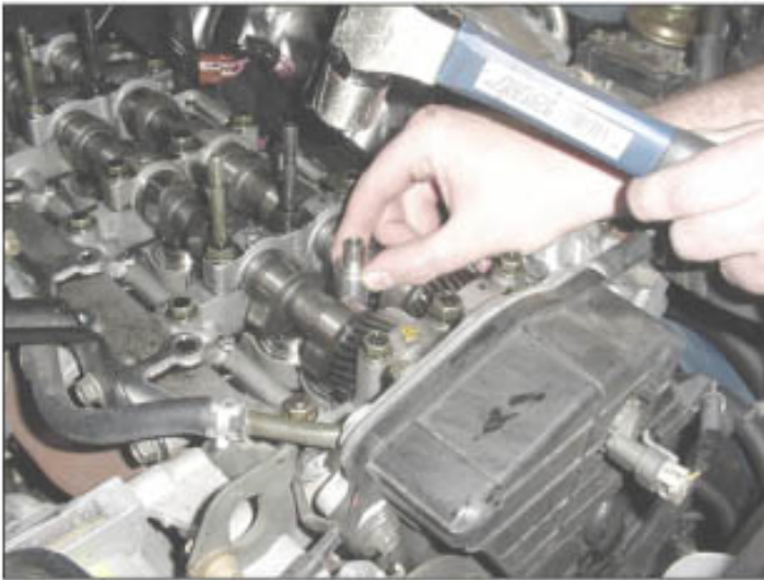
Figure 13 – Installing new injector sleeve
