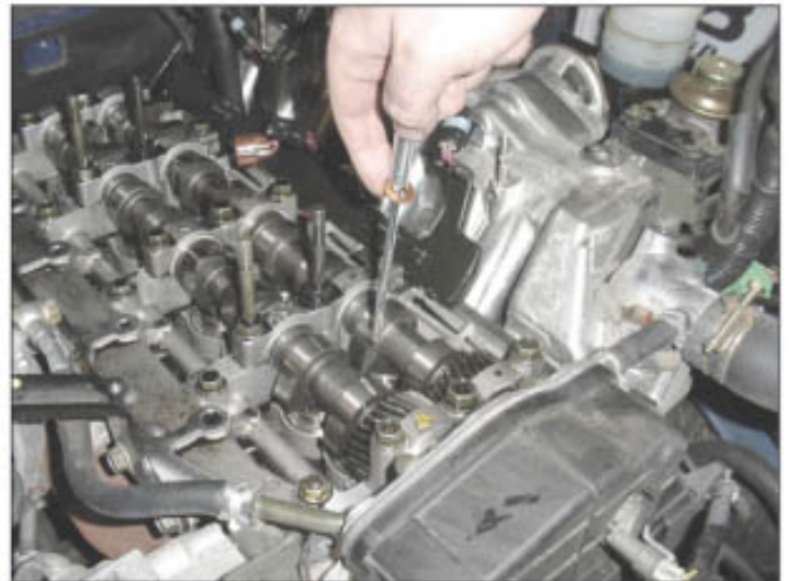
Figure 15 – Installing the copper packing
