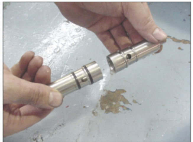
Figure 11 – Using old sleeve as installing tool
