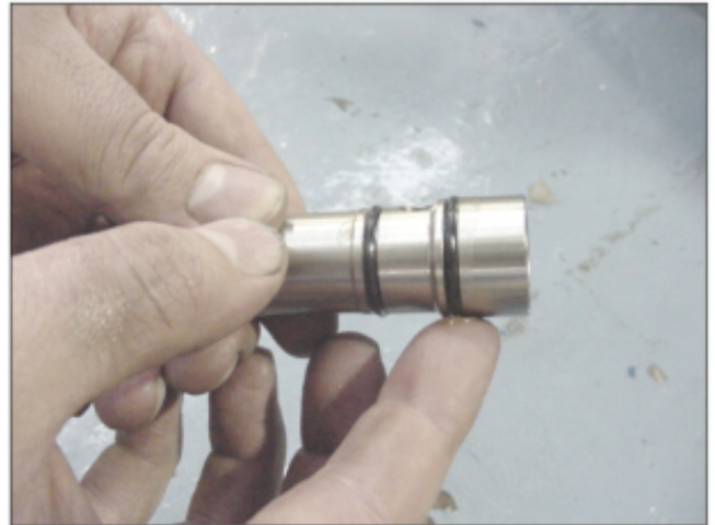
Figure 10 – Greasing new injector sleeve O-rings
